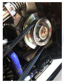
**Buses' Air Conditioning Electromagnetic Clutches**
